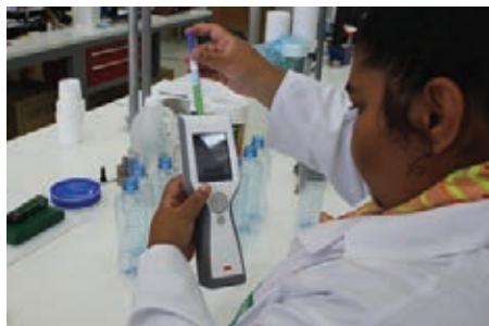
Rapid hygiene testing is done by ATP bioluminescence tests. Results can be obtained in less than 2 minutes.
