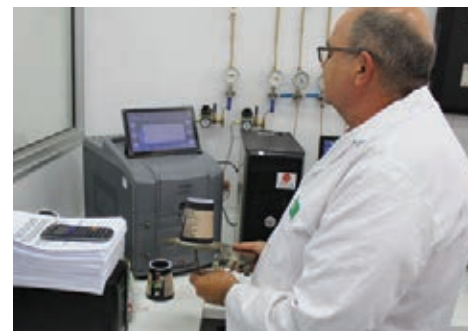
Testing the oxygen barrier of an in-mould labelled tub using our state-of-the-art OX-TRAN machine.
